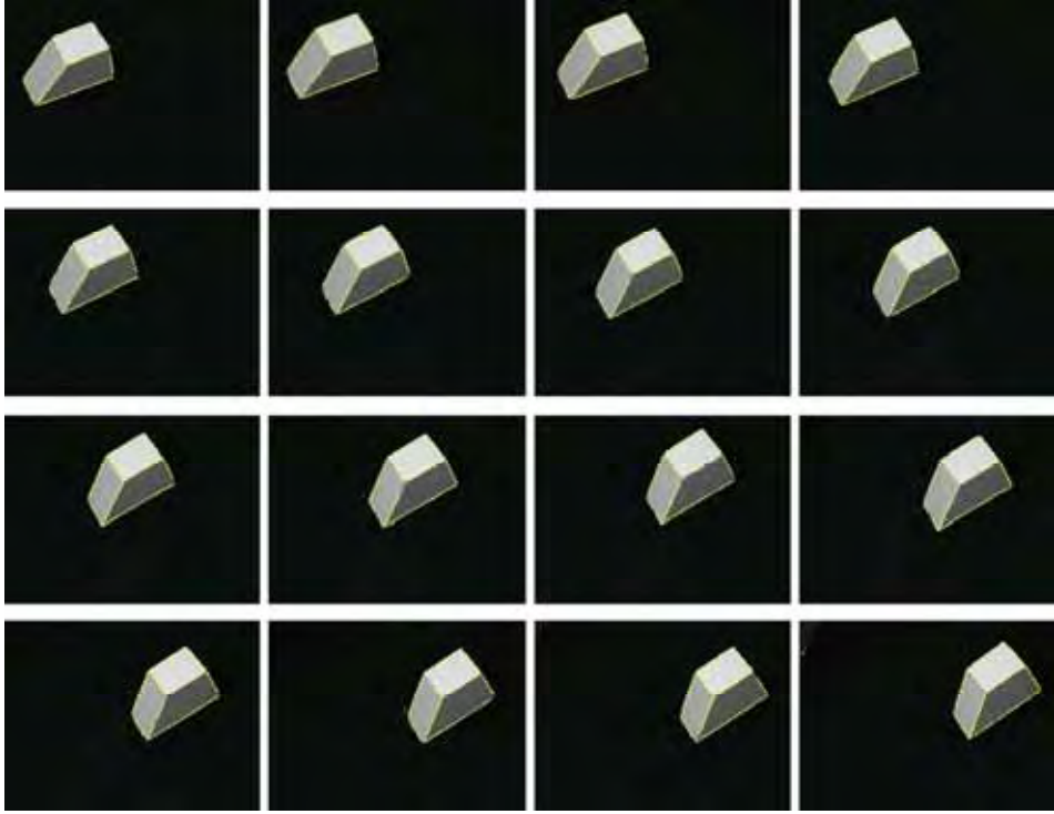
Figure 3. Tracking simple shape in a structured environment. The modelbased polyedral object pose estimation is used to compute the camera displacements during the image sequence
