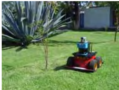
Fig. 1. XidooBot, a Pioneer 3AT robot used as our experimental test bed.
