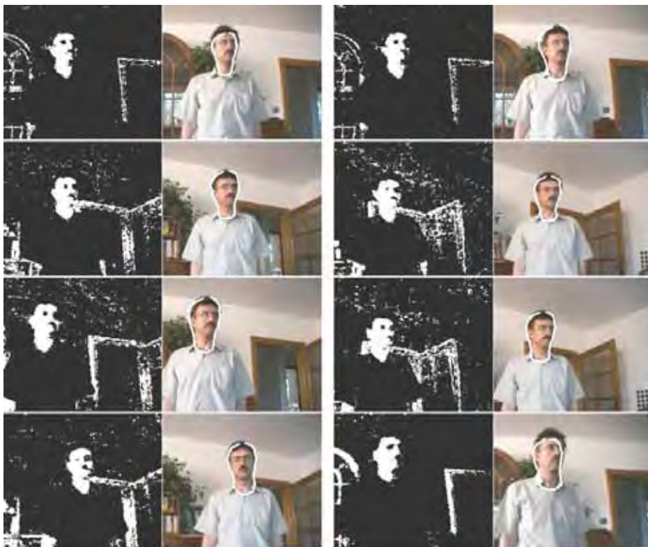
Fig. 4. ASM-based face tracking, using gradient. Frames #1, #2, #20, #60, #80, #100, #120.
