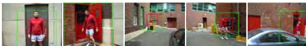
Figure 4. ABCshift successfully tracks throughout the sequence and is not distracted by red regions of background, despite being initialised in image 1 which contains no red background. Frames 1, 176, 735, 1631, and 1862 shown. Green and red squares indicate the search window and estimated object size respectively. This movie, PeopleTracking1ABCshift.avi, can be viewed at the project website (see references).
