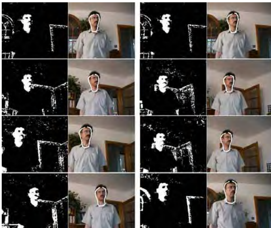
Fig. 9. ASM-based face tracking using the distance to the edge of face mask, intensity gradient and coherence of the phase. Frames #1, #2, #20, #40, #60, #80, #100 and #120.
