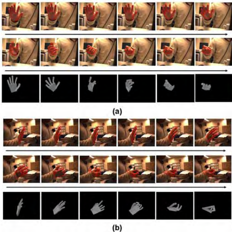
Figure 19. Tracking result by two cameras. (a) Camera 1 view. (b) Camera 2 view.
