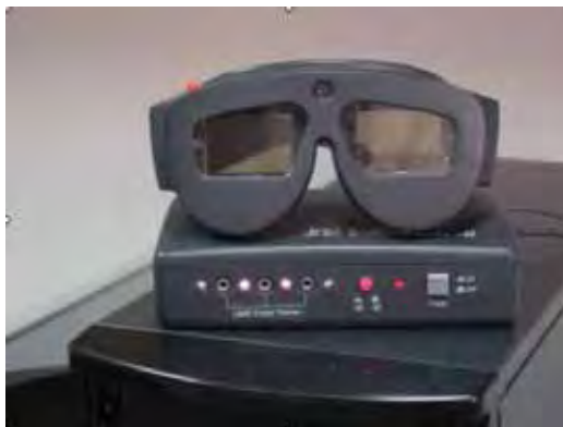
Figure 8. An active infrared control stereo display device and a pair of liquid crystal eyeglasses
