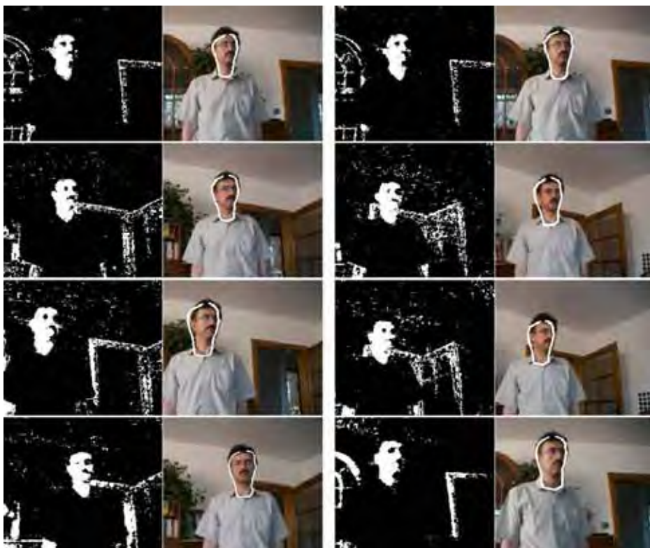
Fig. 5. ASM-based face tracking using intensity gradient and color. Frames #1, #2, #20, #40, #60, #80, #100 and #120.
